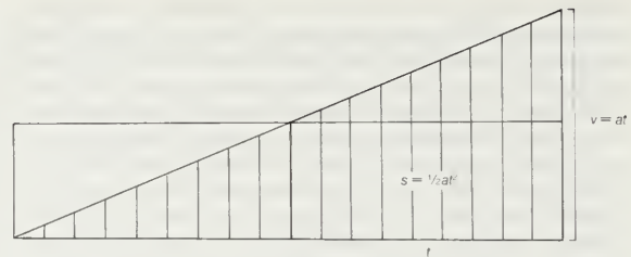
Figure 11: Uniformly accelerated motion; s = speed, a = acceleration, t = time, and v = velocity.
